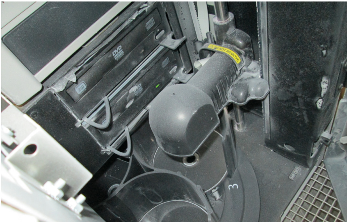
Rimage Catalyst® system with filtered positive air flow
